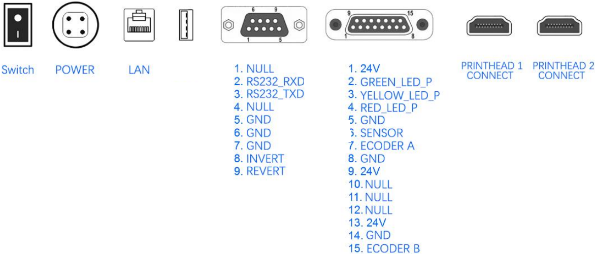
Figure 3-2 T220E Online inkjet thermal inkjet printer external interface
